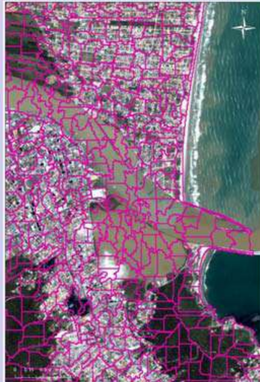
(left) Detail of the reconstructed TWL from the SSDs (blue dots) . (right) Detail of the configured cells in the RFMS model.
