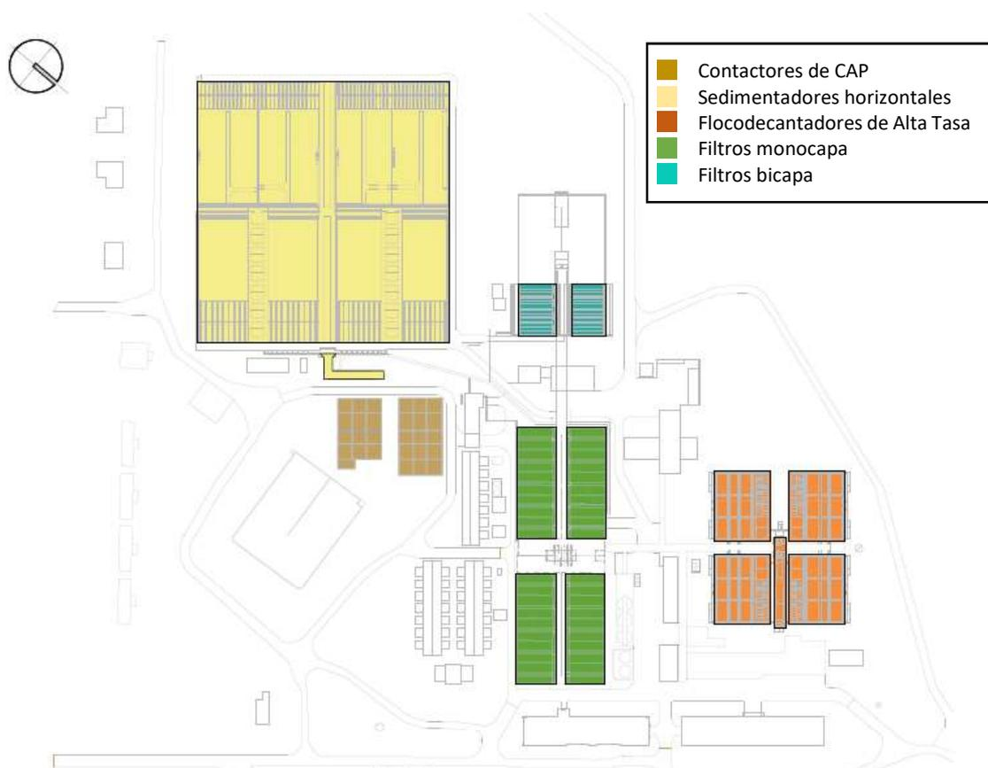
Figura 2-5: Planta General Planta Aguas Corrientes.
