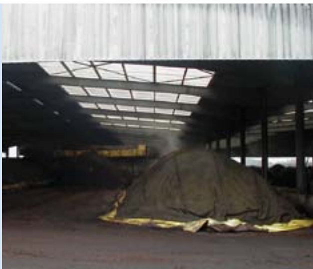
Intensive rotting under a semi-permeable membrane
