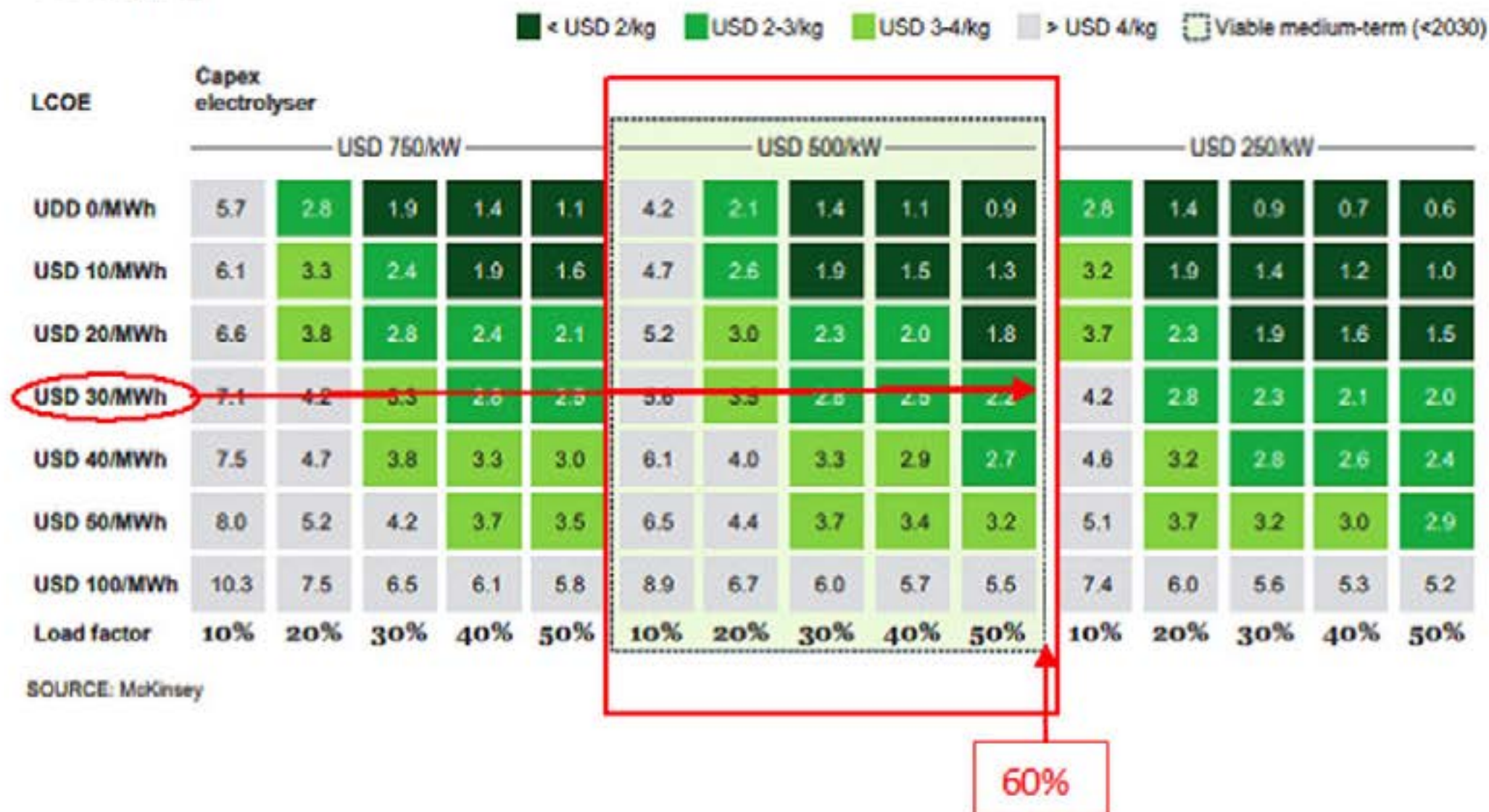
Cost of renewable hydrogen with varying LCOE and load factors USD/kg H 2
