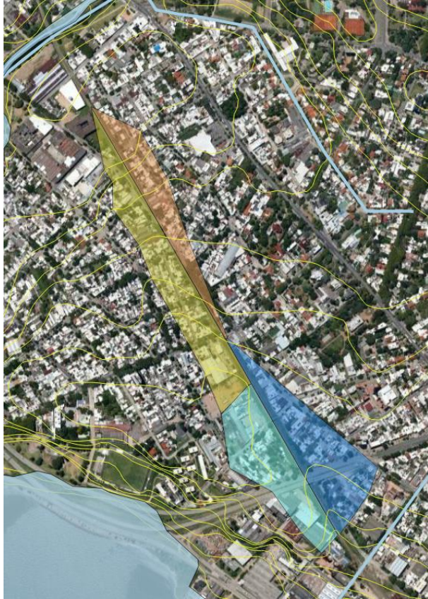
Figure 5-7 Montevideo trench surface runoff catchments
