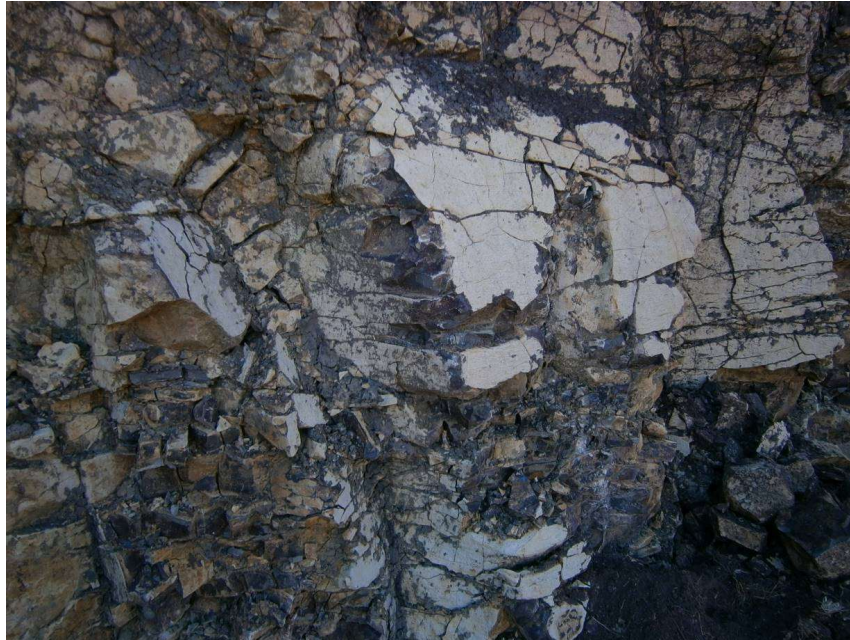
Figure 9. Fine to medium grained Basalts, in front of quarry next to the railroad
