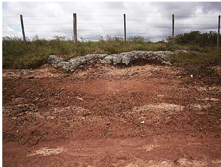
Figure 7. Residual soil profile developed from Formation Mercedes sandstones
