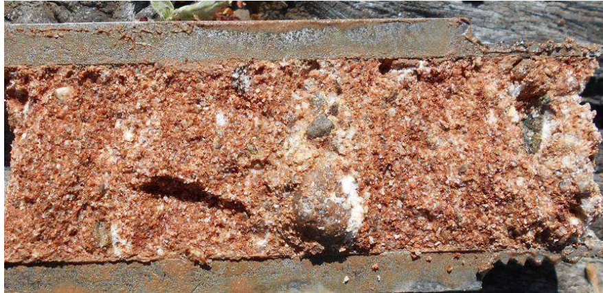
Figure 6. Sample of coarse sand thick with boulders, recovered in the test SPT sampler
