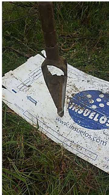
Figure 13. Rotating manual drilling tool used in soundings points
